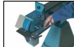
Belt travel adjustment - Easy to adjust.
