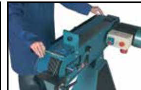
Tool free quick belt change - Without removing guards.
